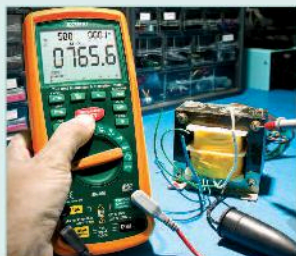
Measure the insulation resistance of transformer windings
